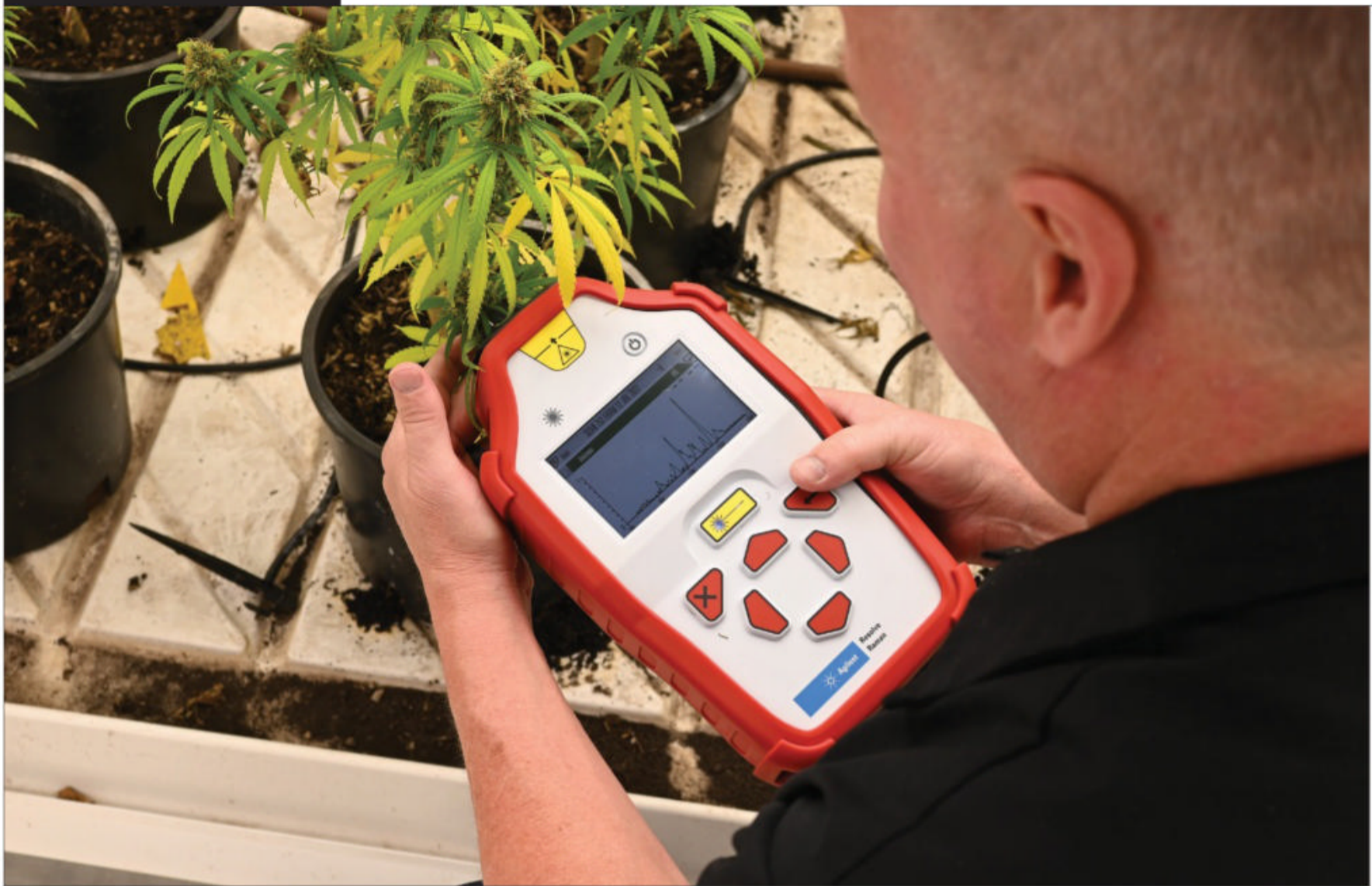
AGILENT'S HANDHELD LASER-OPERATED SPECTROSCOPY TOOL AT WORK.
